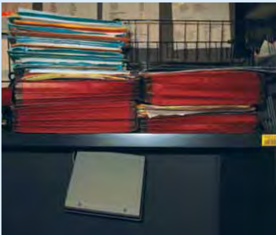
An RFID sensor under a work surface automatically checks files out to the person who works there.
