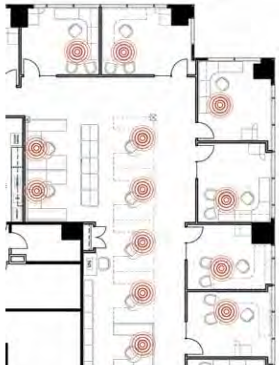
RFID sensors in cubicles and offices automatically track files as they move.
